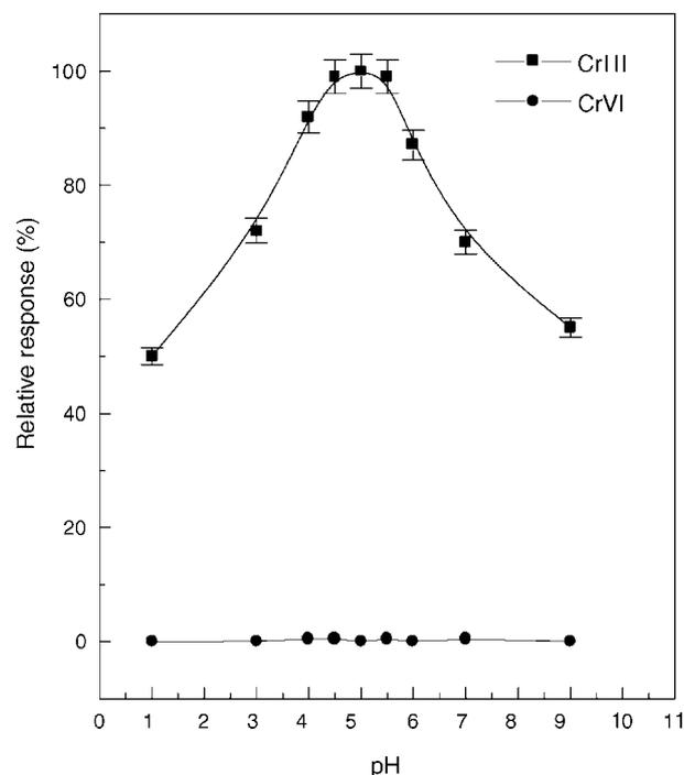
Fig. 2. Dependence of Cr(III) and Cr(VI) retention on pH of loading solutions. Preconcentration of 10 ml of Cr(III) and Cr(VI) solutions; chromium concentration was  $0.5 \mu\text{g l}^{-1}$ ; nitric acid concentration was 1.0% (v/v).
