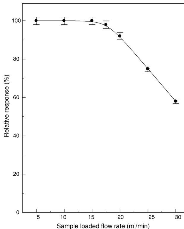
Fig. 3. Dependence of recovery of metal on sample flow rate. Preconcentration of 10 ml of Cr(III) and Cr(VI) at pH 5.0; chromium concentration was  $0.5 \mu\text{g l}^{-1}$ ; nitric acid concentration was 1.0% (v/v).
