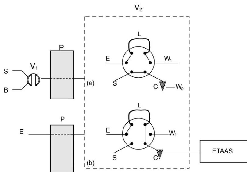
Fig. 1. Schematic diagram of the instrumental set-up. S, sample (flow rate: 15.0 ml min<sup>-1</sup>); B, buffer; E, eluent (flow rate: 0.2 ml min<sup>-1</sup>); L, loop 50 µl volume; W<sub>1</sub>, W<sub>2</sub>, wastes; P, peristaltic pump; C, minicolumn packed with activated carbon; V<sub>1</sub> and V<sub>2</sub>, injection valves. Valve positions: (a) sample loading; (b) injection.
